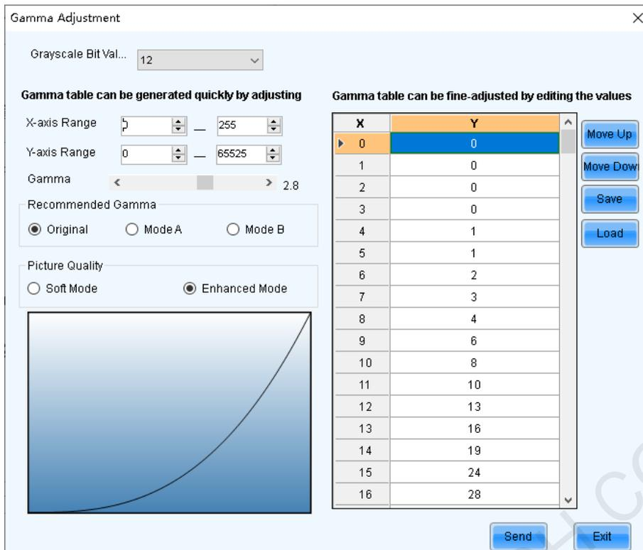
Step 3 Perform any of the following operations as required to configure the Gamma curve.
