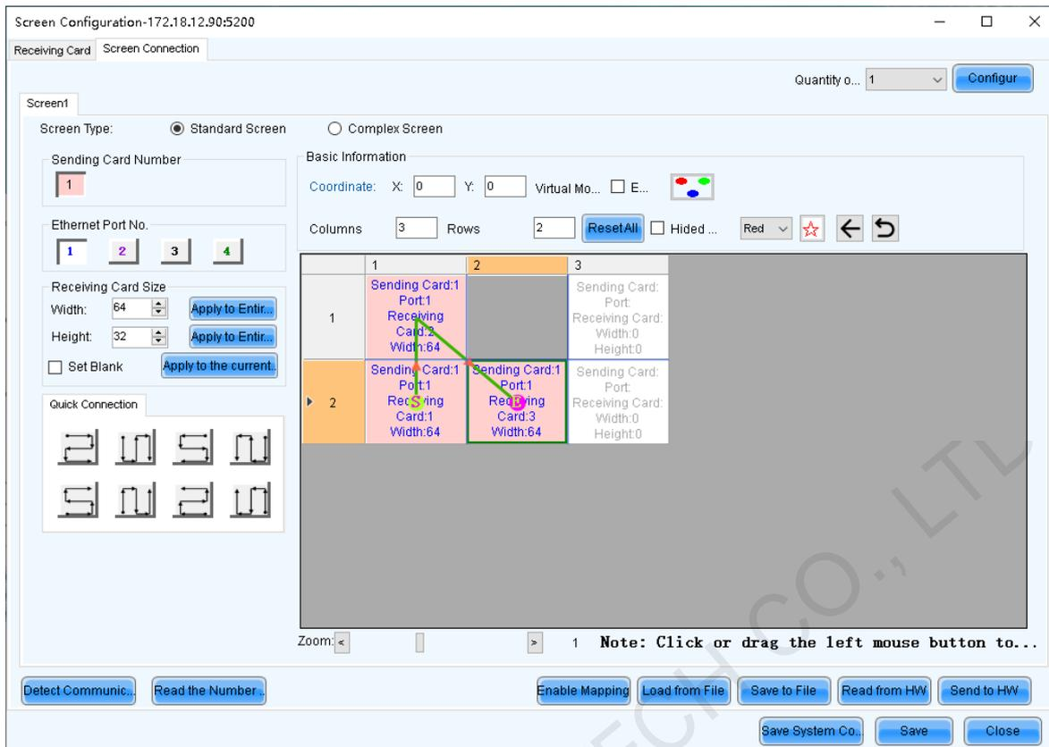
Step 7 Repeat Step 4 to Step 6 to set the receiving cards loaded by the other output ports.
