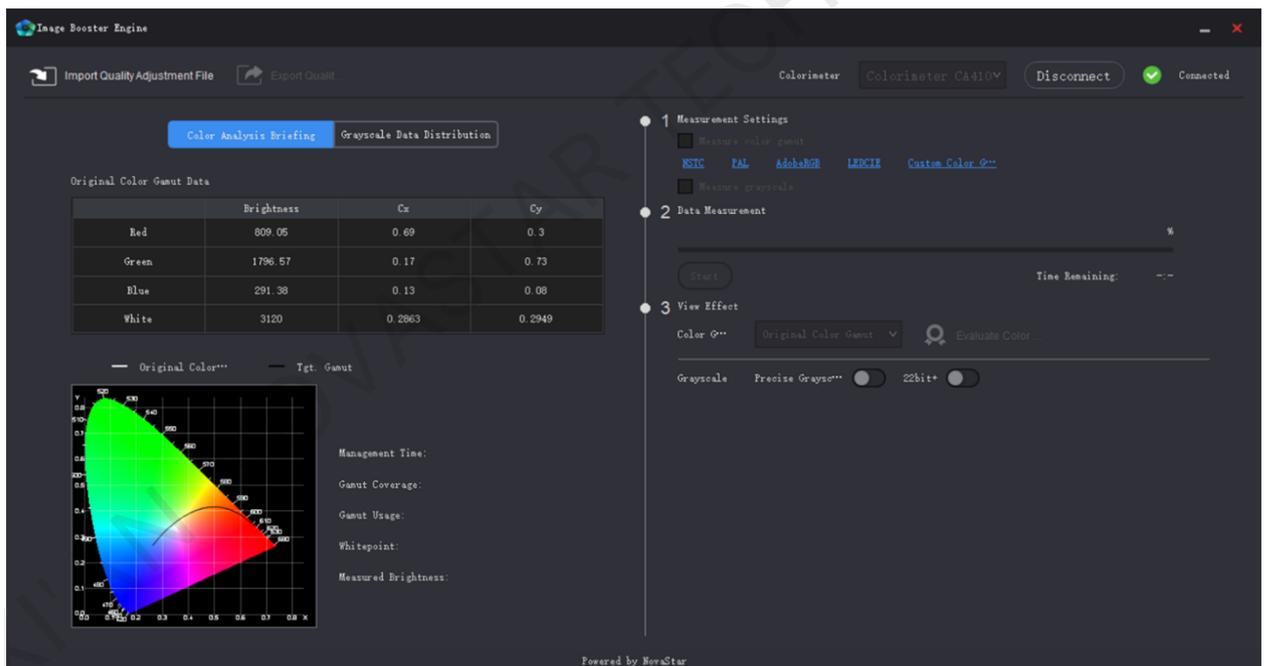
NovalCT will connect to the colorimeter automatically. If you see
