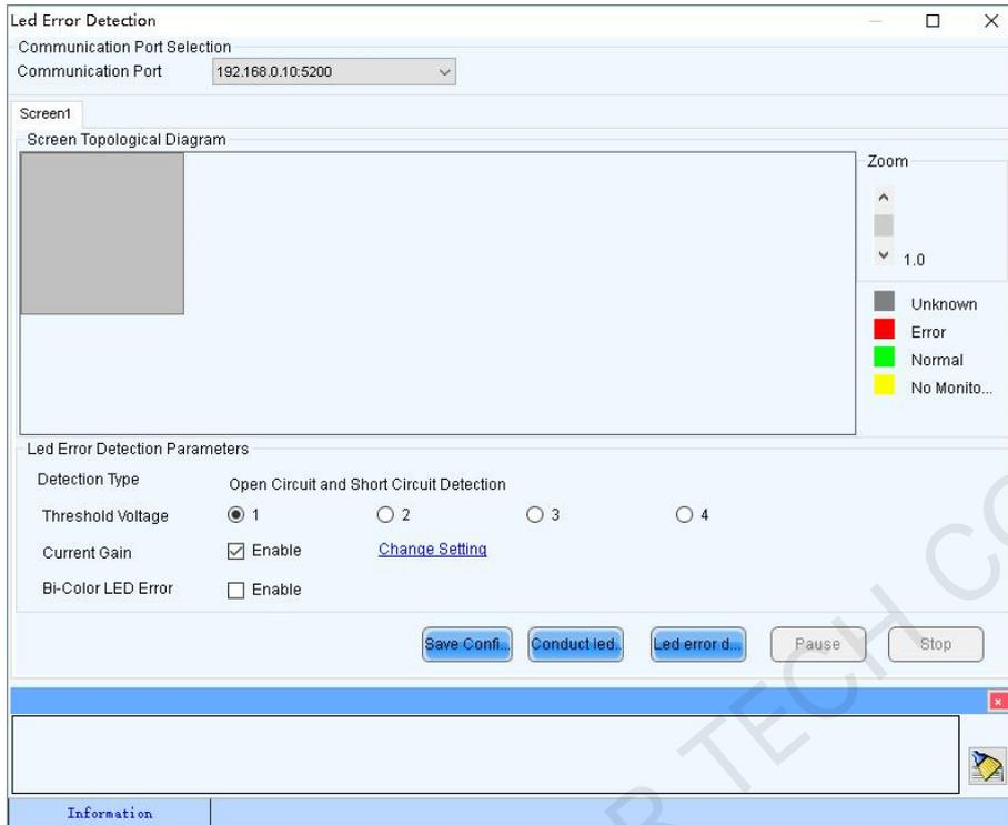
Step 3 Set Led error detection parameters.
