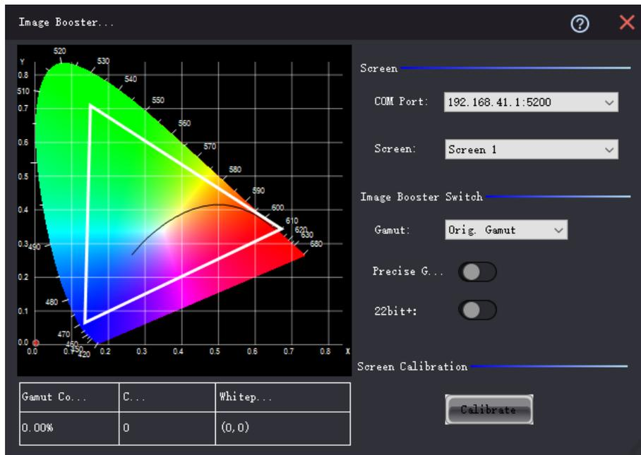
Step 4 Select a color gamut, set the precise grayscale and 22bit+ switches, and view the effect on the screen.
