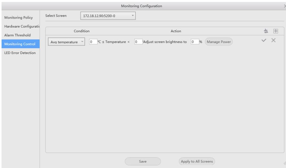
Set the rules for automatic control of average temperature, maximum temperature, smoke and backup power supply. If the control type is set to smoke, a multifunction card must be configured in advance. After the settings are done, click **Save** or **Apply to All Screens**.
