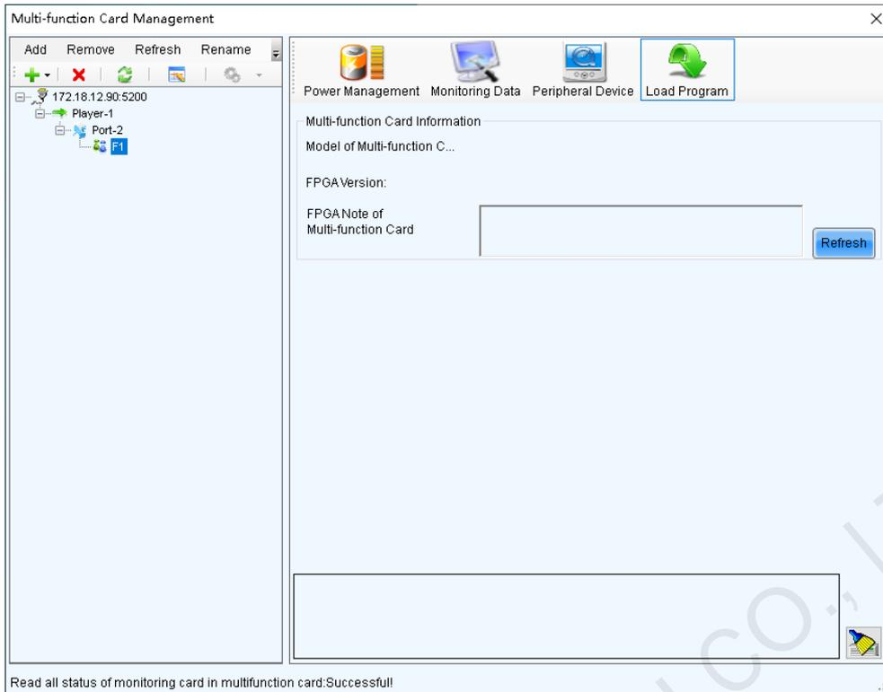
Click **Refresh** to view the multifunction card model, FPGA version and FPGA note.
